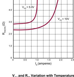
On-Resistance vs. Drain Current
